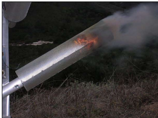
Figure 4 Flare burning inside spark arrester
