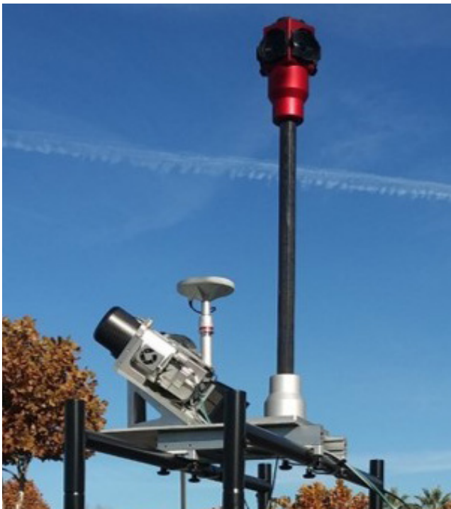
RIEGL VMX-2HA High Speed, High Performance Dual Scanner Mobile Mapping System
