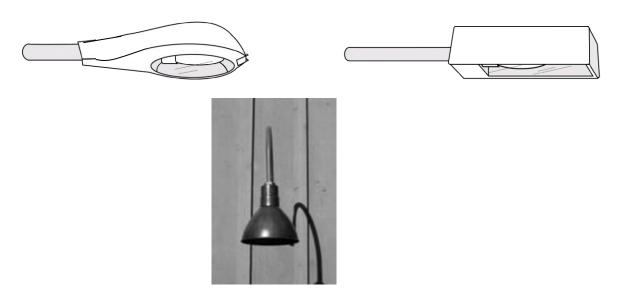
2. <u>Partially Shielded Light.</u> An outdoor light fixture that may allow some light to pass through a semi-translucent barrier, and/or may allow visibility of the lamp from certain perspectives.
