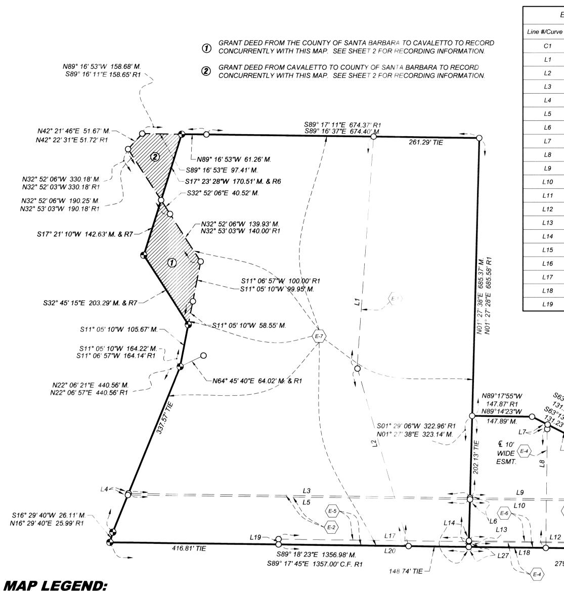
BASIS OF BEARINGS: A MEASURED LINE BETWEEN TWO FOUND SURVEY MONUMENTS AS SHOWN ON SHEET 2.
