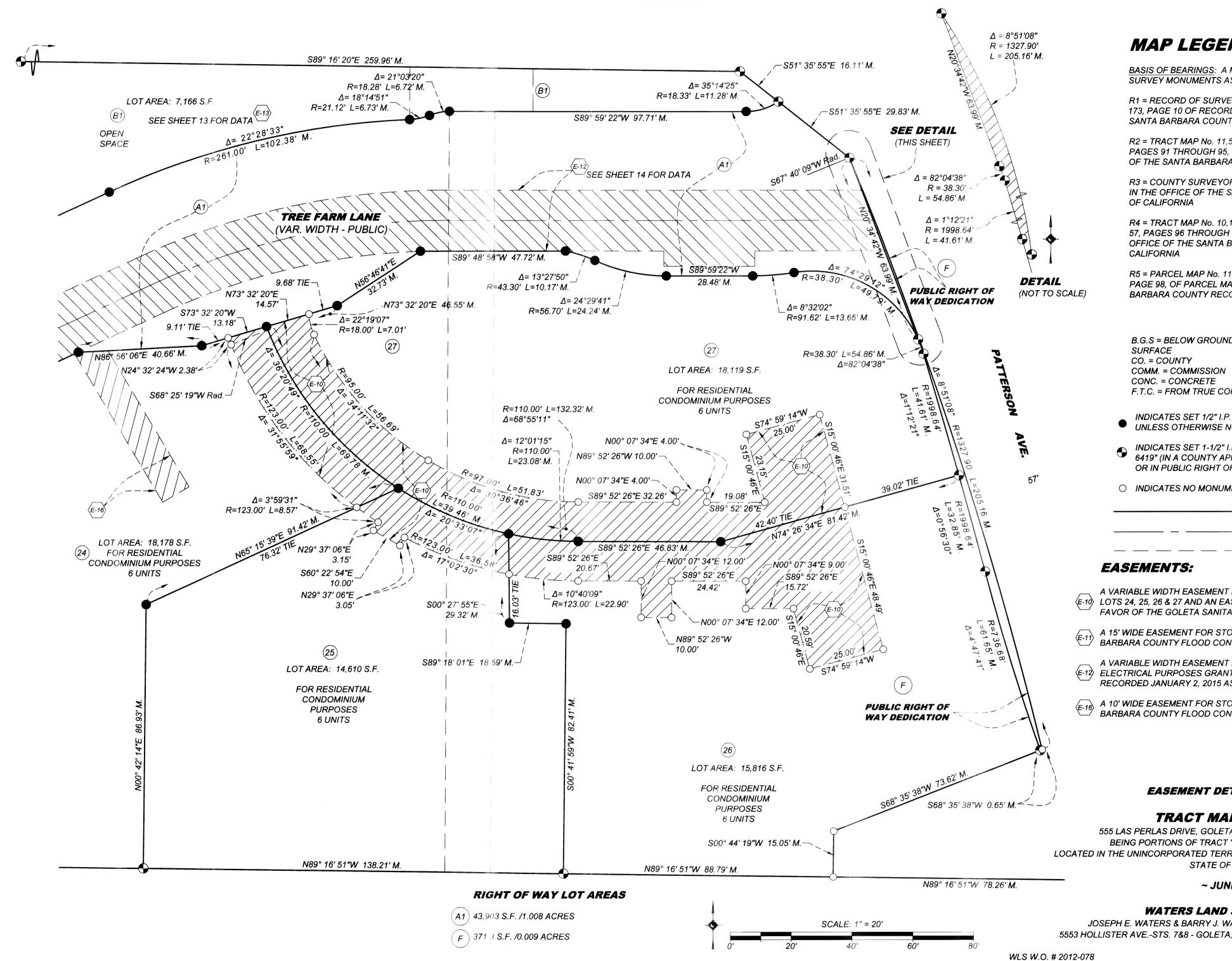
BASIS OF BEARINGS: A MEASURED LINE BETWEEN TWO FOUND SURVEY MONUMENTS AS SHOWN ON SHEET 2.
