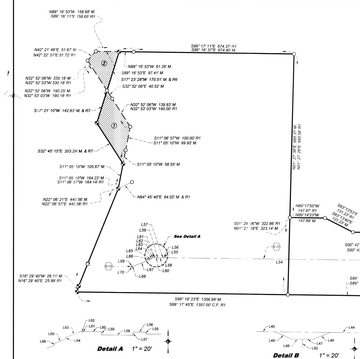
BASIS OF BEARINGS: A MEASURED LINE BETWEEN TWO FOUND SURVEY MONUMENTS AS SHOWN ON SHEET 2.
