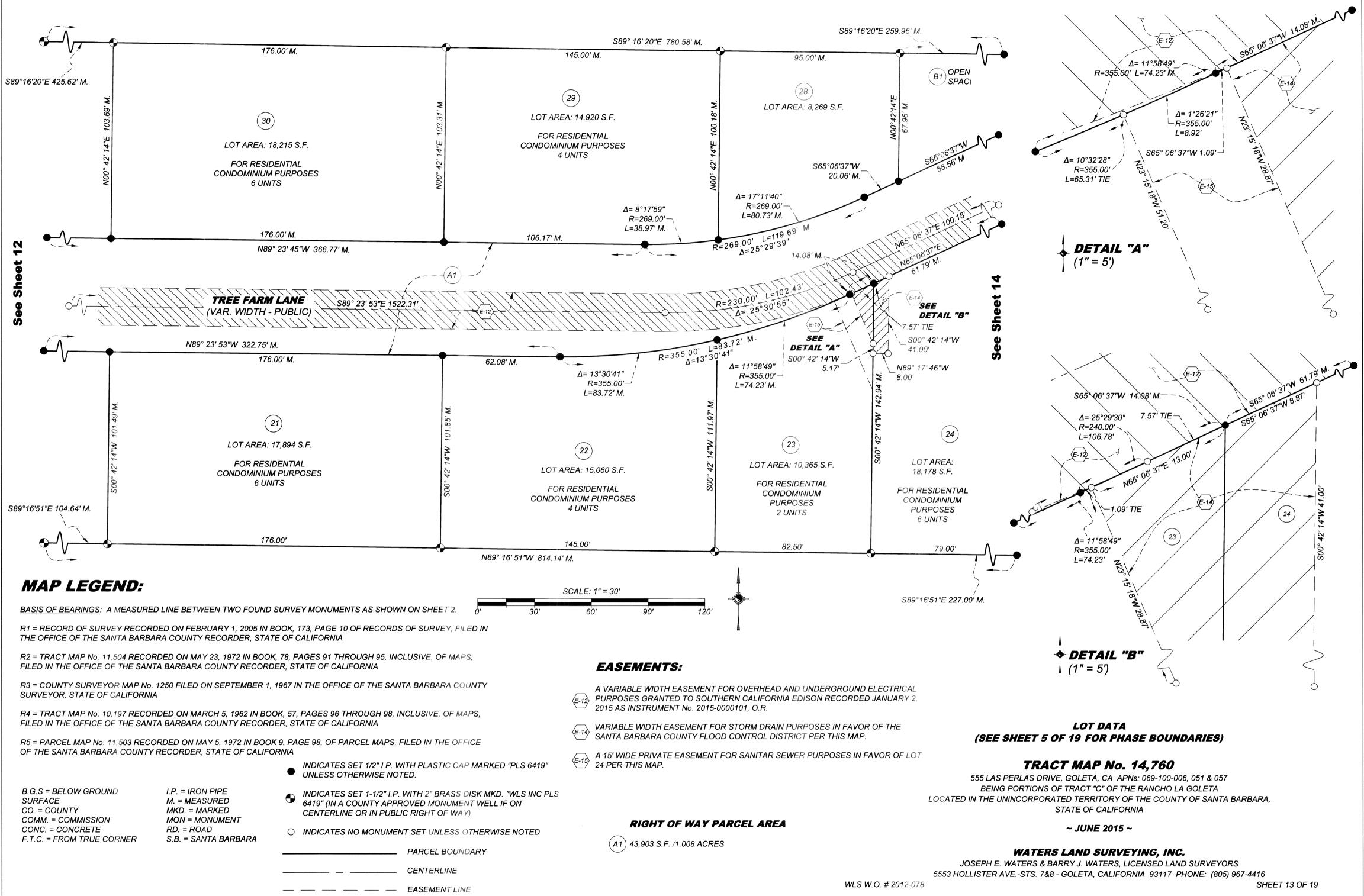
BASIS OF BEARINGS: A MEASURED LINE BETWEEN TWO FOUND SURVEY MONUMENTS AS SHOWN ON SHEET 2.
