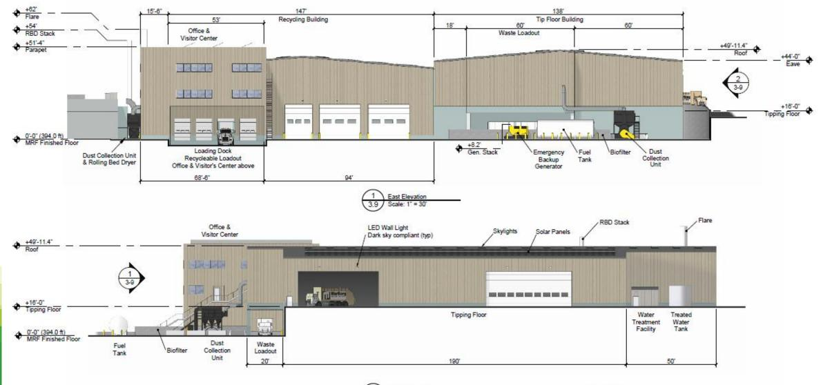
2 North Elevation 3.9 Scale: 1" = 30' Abbreviations RBD = Rolling Bed Dryer
