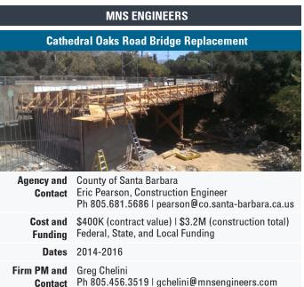
**Objective.** This \$3.2M project replaced the existing bridge spanning over San Antonio Creek on Cathedral Oaks Road with a single-span, pre-stressed, box girder bridge on cast-in-drilled-hole (CIDH) piles. The bridge is located at a major arterial intersection and at the entrance to Tuckers Grove Park. Due to this high volume of activity, daily traffic control and coordination with the public was required.
