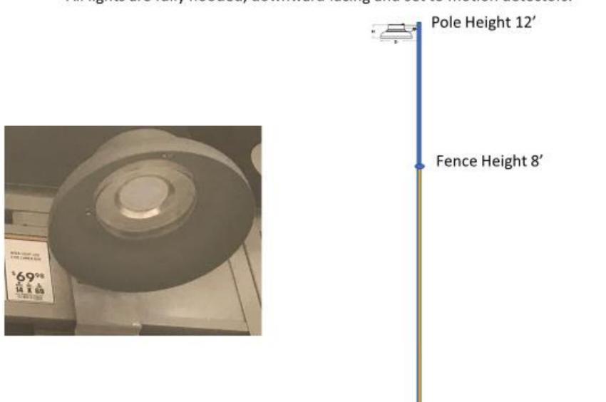
All lights are fully hooded, downward facing and set to motion detectors.
