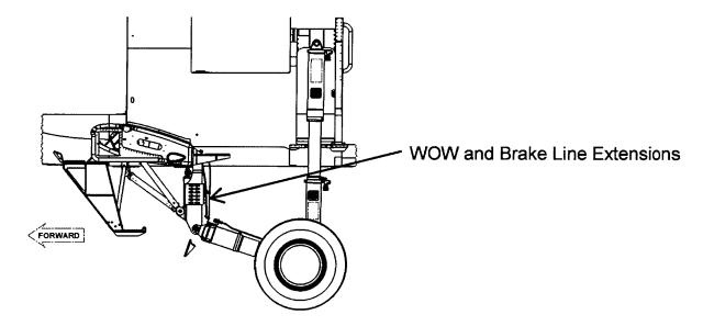
**b)** The aircraft sits on the ground with the nose up 3.6 degrees. In this configuration three gearbox oil level indicators are adjusted accordingly. The main transmission dip stick is etched with new Add/Full markings.
