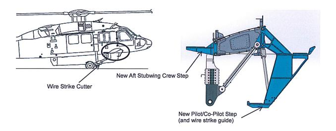
The addition of the two stubwing steps requires a modification to the stubwing fairings. Two areas of the stubwing fairing are removed to allow proper clearance for the step attachment structure.
