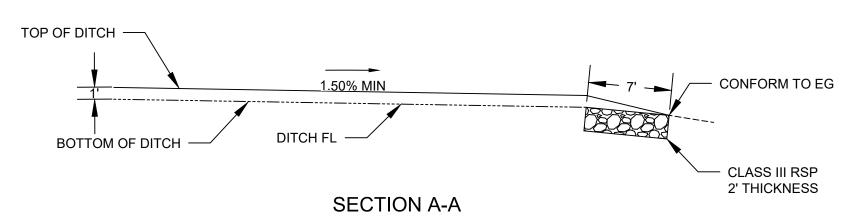
RSP AT DITCH OUTFALL DETAIL NOT TO SCALE
