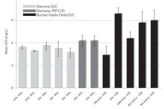
**Figure 1.** Mean DO values during crushing operations. Error bars = 1 sd (mh: machine harvested D/C: destemmer-crusher C/D: crusher-destemmer)
