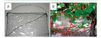
Figure 1. Vineyard trap for airborne 1,8-cineole fashioned out of 20 cm  $\times$  30 cm polypropylene sheet and wire mesh (A) and traps installed in the grapevine canopy (B) in vertical (left) and horizontal (right) positions.
