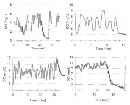
**Figure 2.** Real-time DO profiles during crushing at the JCW. DO (dynamic) light grey, DO (static) dark grey. Clockwise from top left: machine harvested (MH) Pinot Noir; MH Sauvignon Blanc; MH Riesling; handpicked Riesling. Vertical bars on the time scale indicate pump on, crosses pump off.
