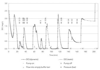
**Figure 3.** DO profile during pressing of crushed machine-harvested Riesling (Bucher Xpert 250 with ORTAL program)
