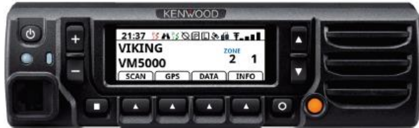
Figure A-1.4-13. Viking VM5000 Mobile Radio Programmable Option Buttons
