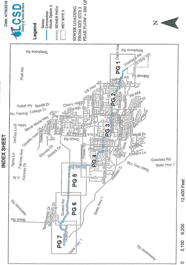
EXHIBIT 3: KEY SITE 3 SEWER MODEL CAPACITY IMPACT ANALYSIS **OPTION 3 - PRESSURIZED FLOW TO NORTH TRUNK LINE**
