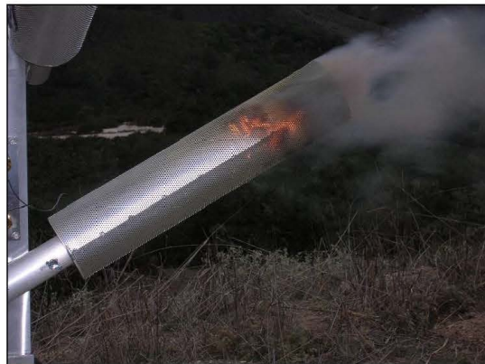
Figure 4 Flare burning inside spark arrester
